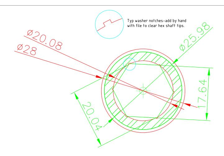
Green hatch shows the available space for a washer. Measurements in green are for hex shaft and ID of sprocket adapter.
