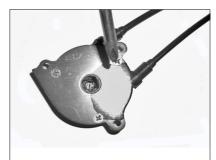
Unfasten the fixing bolts which are fixing the shifting cables by using a 3mm Allen key.
