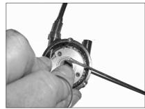
Turn the shifter to position No. 9 and bring the cable in. Run the cable through the casing into the shifting unit. Bring the cable almost one tour around the cable ring. Pull the cable hard and tighten the fixing bolt using a 2.5mm Allen key. Afterwards cut both cables to a proper length and turn the shifter back to position No.1.
