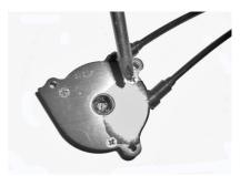
Check if the tension of the shifting cables is adequate. If the tension is to high the shifting will beome to hard. Pull the cabels slightly. You should have 1-2mm space on both sides.
