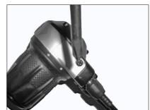
In order to pull out the shifting cables you have to put the shifter to gear No. 3......
