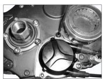
Take off the shifiting unit (No. 9 page 1) using a 3mm Allen key.
