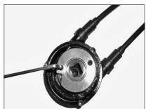
Take off the cover plate by using a Phillips screwdriver No. 2
