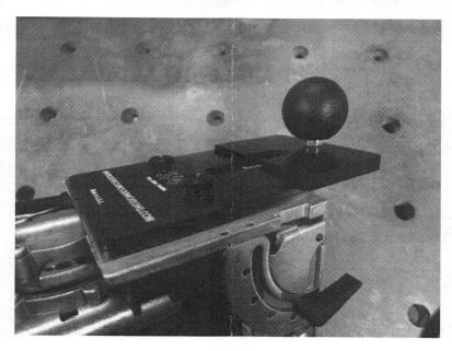
Using the Domino plate allows you to locate your mortises using pencil marked lines, the paddles or pins (depending which model Domino you own) or the Festool # 493488 Cross Stop attachments.
