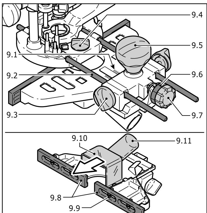
The parallel guide (accessory) can be used for routing parallel to the edge of the workpiece.
