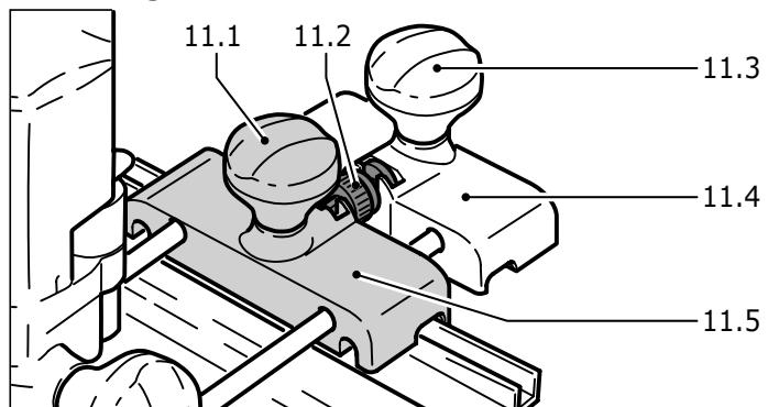
The distance X (fig. 10) of the router to the guide rail can be set finely using the fine adjustment (Accessories).
